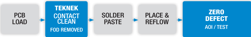
Figure 1: FOD removal sits ahead of solder paste print — the single most consequential point in the line to intercept it.
