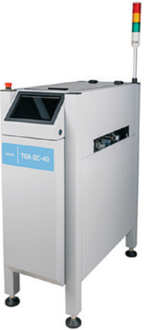
Teknek's Tek-BC 40 inline board cleaner, positioned ahead of solder paste print.
